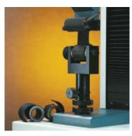
Fig 17. Checking the peeling strength of the outer layer of rubber hose, using a combination of standard and custom grips
