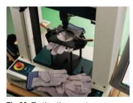
**Fig 30.** Testing the puncture resistance of work gloves
