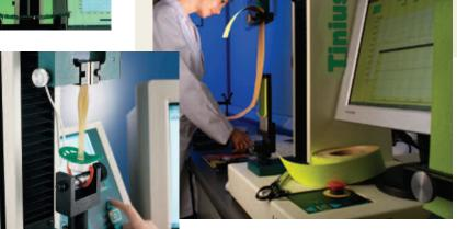
Fig 9. A model H5kT and a model H5kS being used to determine the bonding strength of adhesive tape
