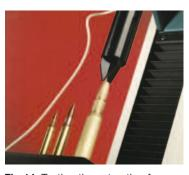
**Fig 14.** Testing the extraction force of a bullet from its cartridge using custom pneumatic grips
