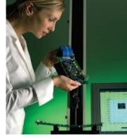
Fig 8. Model H1kS being used to find the tensile strength of a baby's pacifier
