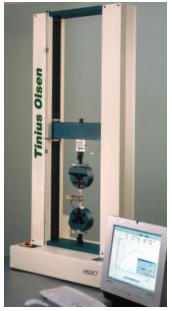
Fig 37. Model H50kT with HT21 grips
