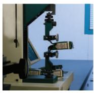
**Fig 11.** Testing the strength of coffee packaging using the quick release vise grips, HT55
