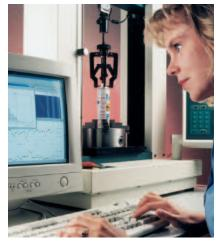
**Fig 39.** Testing the tensile strength of the seam on a shaving foam canister
