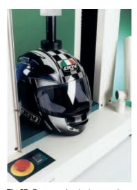
Fig 27. Compression test on crash helmet
