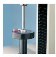
**Fig 15.** Testing the crushing strength of pills
