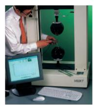
Fig 23. Dumbbell sample of sheet metal being tested with HW21 grips
