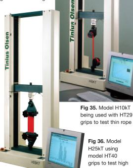
Fig 36. Model H25kT using model HT40 grips to test high strength flexible sheet materials
