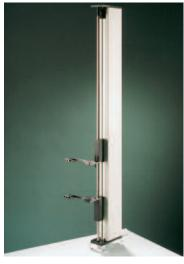
Fig 29. Tinius Olsen high travel extensometer, model 100RC
