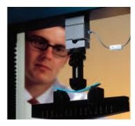
**Fig 24.** A 3 point bend test being performed with model HF72 flexural jig on plastic sample
