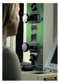
Fig 32. Tear test on rubber specimens
