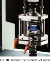
**Fig 18.** Testing the strength of plastic building blocks with a custom attachment
